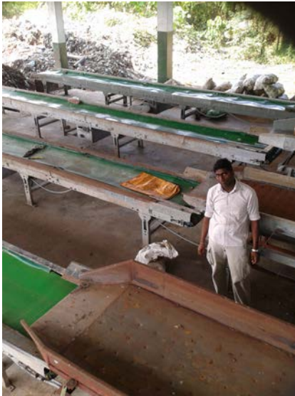
Figure 4.2: Conveyor belts used for waste separation
